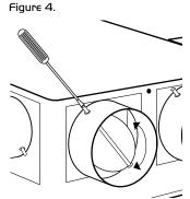
Spigots and spigot blanks are easily removed.
