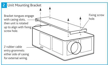
It is also assumed that compatible ductwork is already installed and ready to be connected to the 125mm diameter discharge and inlet spigot.
